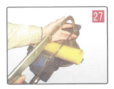
4. Shorten the plastic shield tubes one at a time by cutting the same length that was cut from the inside drive tubes.
