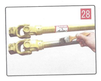
Grease the internal drive tube and reassemble the shielding on the driveshaft.
