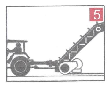
The tractor must be hitched to the implement and positioned so that the angles of the joints are minimal and equal.
