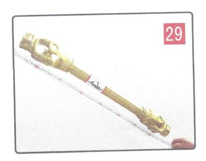
Check the length of the driveshaft in the minimum and maximum positions of the machine. The drive tubes should overlap by 1/3 of their length during working conditions; Shield tubes should never separate while in use.
