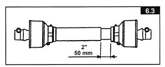
Take particular care when connecting the two Cardan shaft end forks and make sure that they are fully secured. This is achieved by inserting the safety pins and bolts 1 (see pict. 6.4) in the special slots 2 on the power takeoff shafts on both the tractor and machine ends. Use opening on the protective hood (see pict.6.5) to easily fit the shaft end fork with friction disks clutch.
